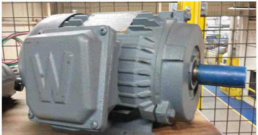
Phase Motor With Cast Iron Housing
