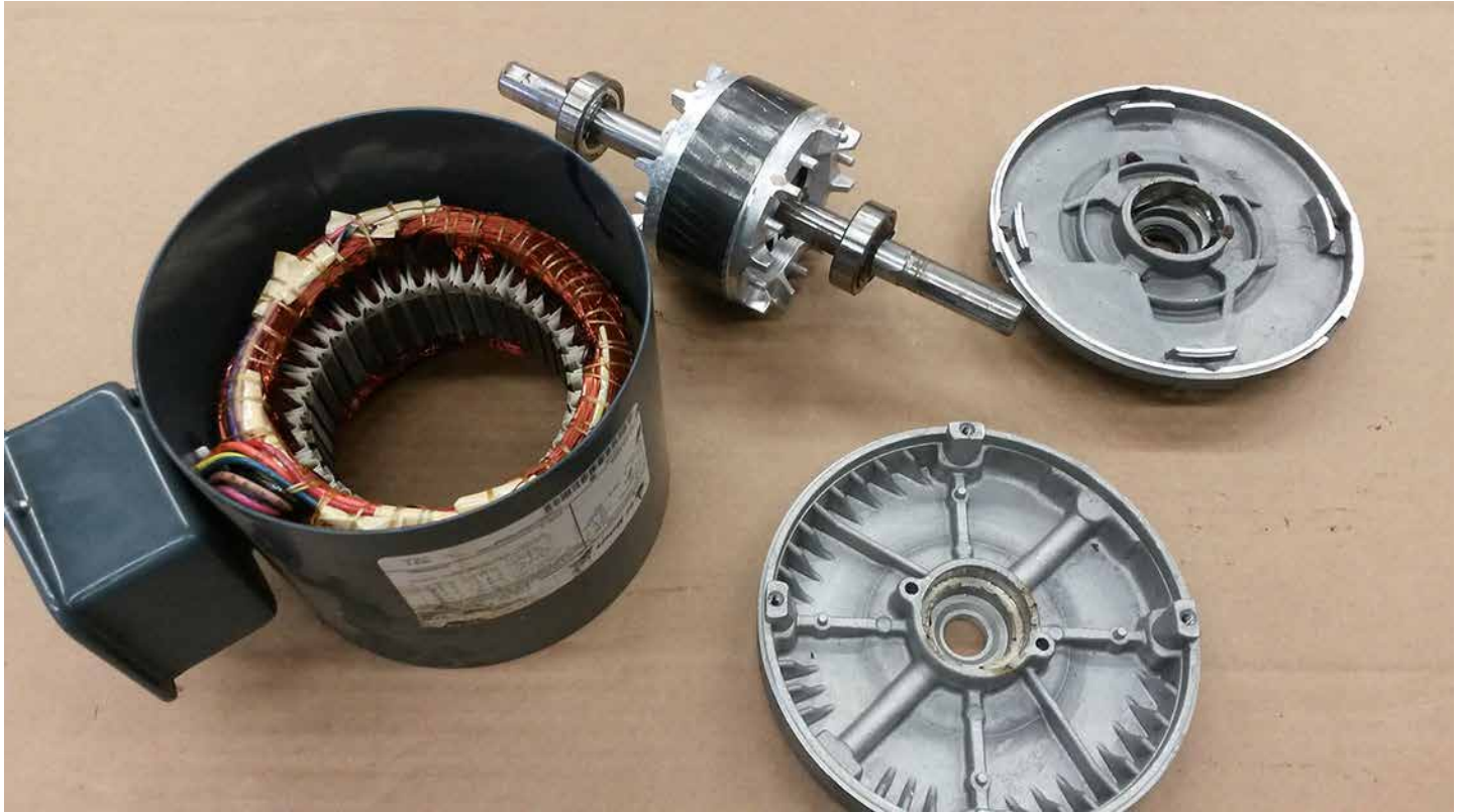
A typical induction motor is disassembled to show its internal components
