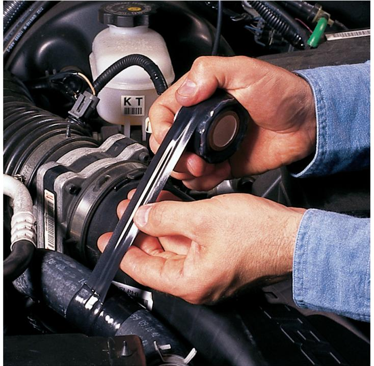
Silicone tape is available in numerous colors, so finding a color to wrap around your outdoor equipment is easy. Wrapping silicone tape around these parts protects the metal from the elements, prevents the start or spread of rust, and if you purchase more than one color, allows you to quickly identify equipment.
